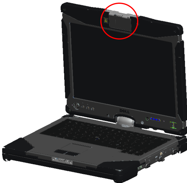
Image above shows the lock in the locked position
